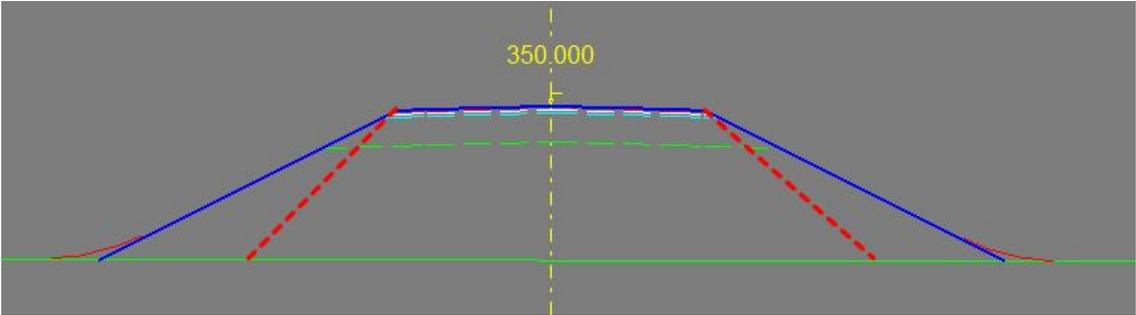
Normally the inner slope starts from the last road surface within surface group 0 to 3, but not always. Cases where the inner slope doesn't start from the last surface we will cover further down this document.
