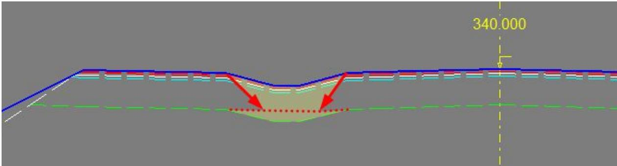
Here the pavement layers for carriageway and bikepath are nearly the same thickness, but it doesn't matter if the bikepath is thinner. The method is still the same.
