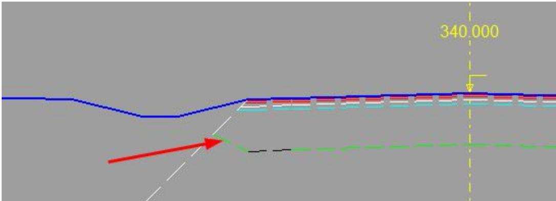
The ending pavement layers will end towards road surface -3.01. This can make some strange results that are handled with a simple Detailed Pavement description.
