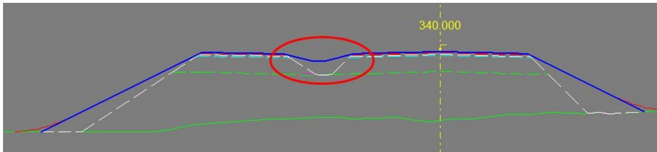
The values in the insert edge function defines how much lateral space the layer needs to be able to be built. The next pavement layer under this use this as a starting point for its own design.
