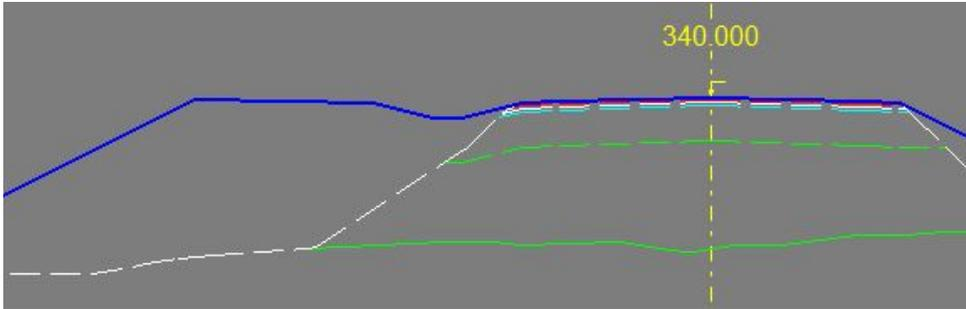
The reason is that we still have pavement descriptions further away from the alignment, after the inserted edge. In our case we want the inserted edge to go back to full pavement for the walk/bikepath, the inserted edge need another 'Insert edge' to work against. You can think in the way that they need to work in pairs, so we have to add the other one.
