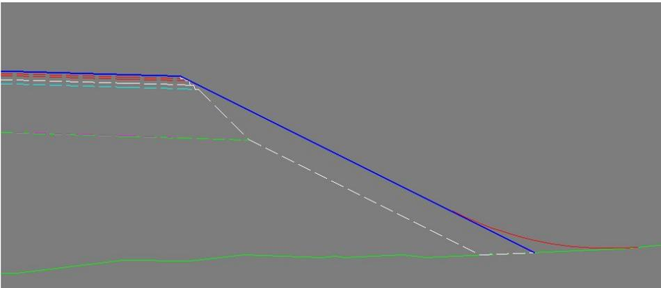
Or if you “don’t want” an inner slope for the pavement layers, but only for the supporting fill, you do as follows: Apply an insert edge with width 0.000 and slope as the embankment slope -0.500. The Insert Edge will “disappear” in the Embankment slope.
